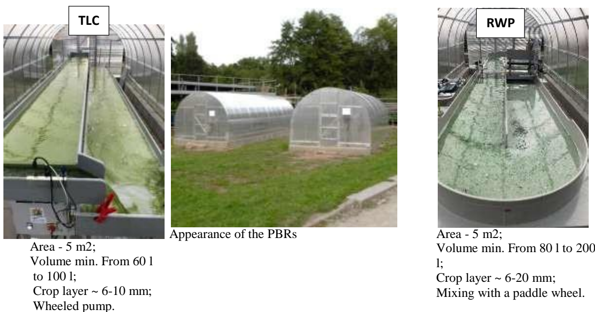
Figure 3 – Cultivation of the Scenedesmus MACC-677 strain in two different PBRs.
